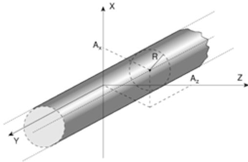
Infinite Elliptical Cylinder || to coordinate axis: **XEC, YEC, ZEC**
