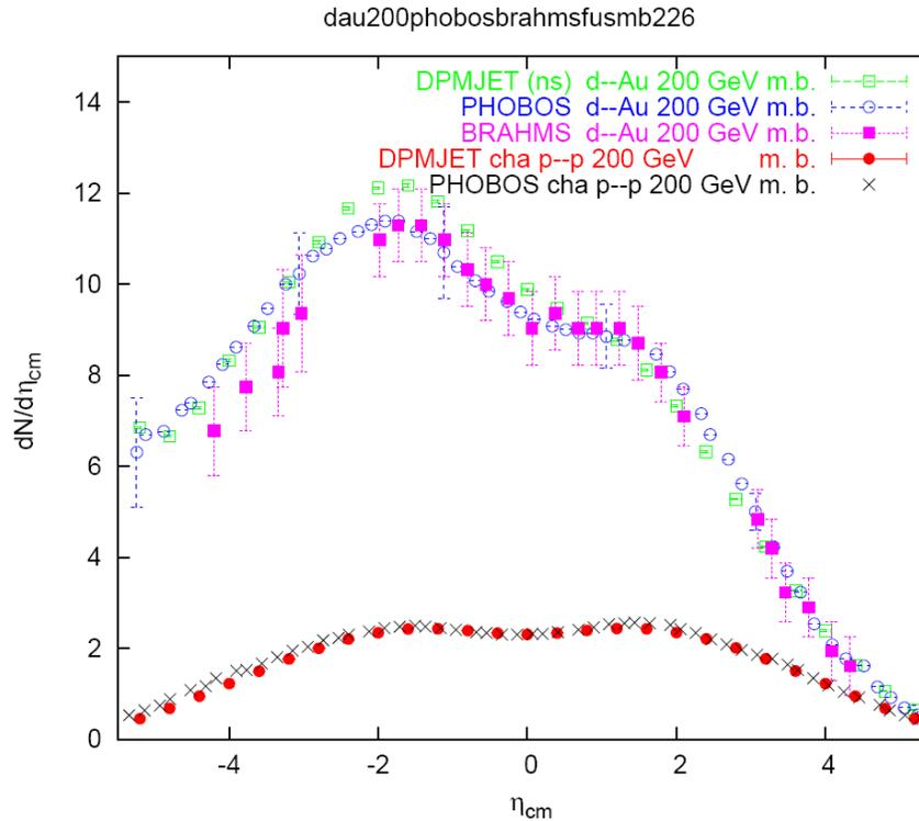
Pseudorapidity distribution of charged hadrons produced in minimum bias d-Au and p-p collisions at a c.m. energy of 200GeV/A.
