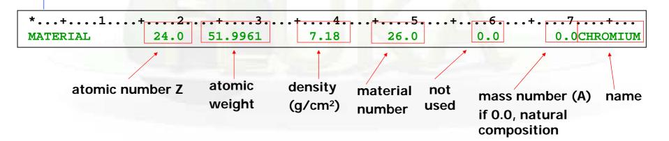
if input is name-based, better leave the material number = 0.0, <u>unless you</u> <u>overwrite a pre-defined material</u> (in that case put the original number)
