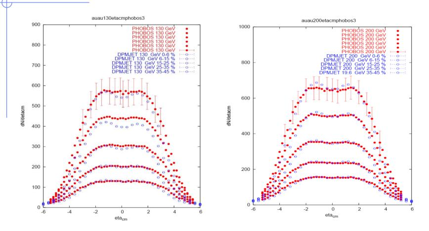
Pseudorapidity distribution of charged hadrons produced in Au-Au collisions at a c.m. energy of 130GeV/A (left) and 200GeV/A (right) for different ranges of centralities.
