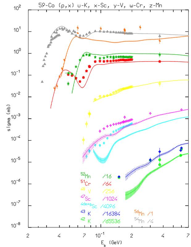
Comparison between computed and measured (A.S. Iljinov et al., Landolt-Börnstein, **Vol. 13a** (1991)) isotope production by protons on natural Cobalt
