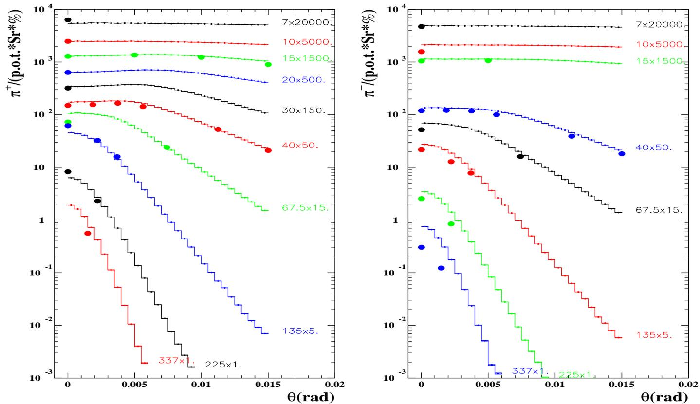
Double differential cross section for  $\pi^+$  (left) and  $\pi^-$  (right) production for 450 GeV/c protons on a 10 cm thick Be target (data from H.W. Atherton CERN 80-07, G. Ambrosini et al. PL B425 208 (1988)).
