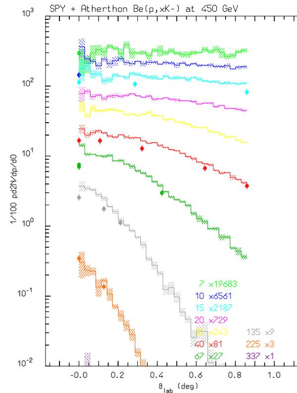
Double differential cross section for  $K^+$  (left) and  $K^-$  (right) production for 450 GeV/c protons on a 10 cm thick Be target (data from H.W. Atherton CERN 80-07, G. Ambrosini et al. PL B425 208 (1988)).
