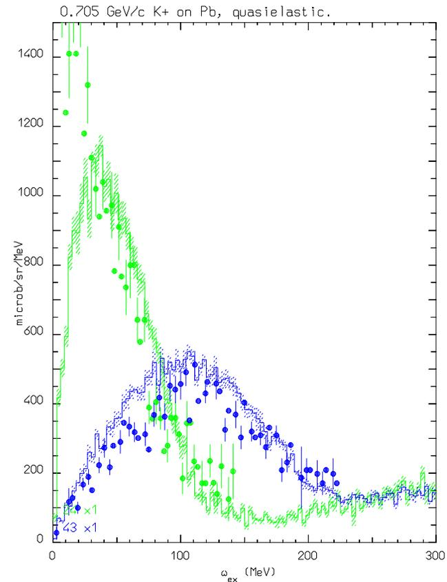
$(K^+, K^{*'})$  on Ca(left) and Pb(right) vs residual excitation, 705 MeV/c, at  $24^\circ$  and  $43^\circ$ . Histo: **FLUKA**, dots: C.M.Kormanyos et al, Phys. Rev. C51, 669 (1995)
