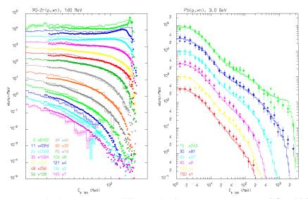
**FIGURE 3.** Emitted neutron spectra at different angles, from 160 MeV protons on Zr (left) and 3 GeV protons on Pb (right). Histograms are FLUKA results, points are experimental data from [30, 31].
