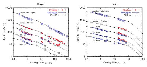
**FIGURE 9.** Dose rate as a function of cooling time for different distances between sample and detector. Left:Copper sample. Right: iron sample, both irradiated at the CERF facility at CERN. Adapted from [42]
