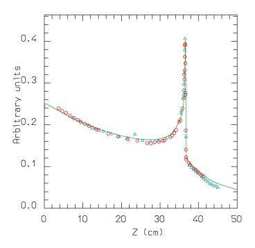
**FIGURE 1.** Dose versus depth distribution for 670 MeV/n  $^{20}$ Ne ions on a water phantom. The symbols represent LBL (circles) and GSI (triangles) experimental data [38], the line is the prediction of FLUKA including the new BME interface. For the profile reproduction at large depths, nuclear interactions below 100 MeV/n play an important role.
