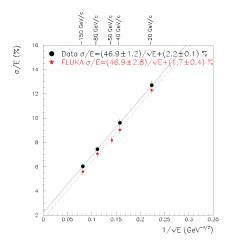
**FIGURE 11.** Fractional energy resolution as a function of beam energy, for a  $\pi^+$ +proton beam at 20°. Experimental data (dots) from [46].
