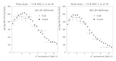
**FIGURE 5.** Computed  $\pi^+$  double differential production cross section for 12.9 GeV/c protons on Aluminum for different angular ranges, compared with experimental data [32].
