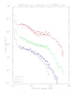
**FIGURE 2.** Emitted proton spectra at different angles, from 160 MeV  $\pi^+$  on a nickel target. Histograms are FLUKA results, points are experimental data from [28, 29]. Note that proton spectra extend up to 300 MeV
