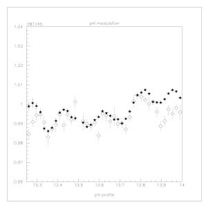
**FIGURE 14.** Modulation of the response of the accordion E.M. calorimeter to a 287 GeV electron beam, as a function of beam impact position. Stars are FLUKA simulations, dots are experimental data. Abscissa values are in  $\phi$  cell units, one cell spanning about 2.5 cm
