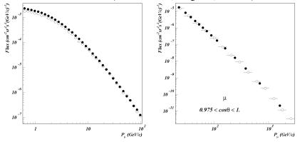
**FIGURE 18.** left: comparison of the simulated  $\mu^-$  flux (open symbols) with the BESS[64] experimental data (full symbols) at Mt. Norikura (2700 m a.s.l.). Right: the comparison of simulated  $\mu^{\pm}$  flux at sea level (open symbols) with the L3+C[65] experimental data (0.975 <  $cos\theta_z$  < 1, full symbols).
