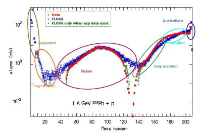
**FIGURE 8.** Residual nuclei production from 1 GeV protons on Lead. Data from [40]
