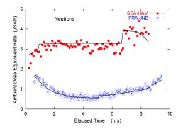
**FIGURE 19.** Ambient dose equivalent from neutrons measured during solar maximum on commercial flights from Seattle to Hamburg and from Frankfurt to Johannesburg, as function of time after take-off (symbols, exp. data, Lines: FLUKA).
