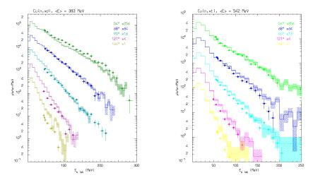
FIGURE 4. Deuteron (left) and triton (right) emission from 383 MeV and 542 MeV neutrons on Cu. respectively (exp data from [27])
