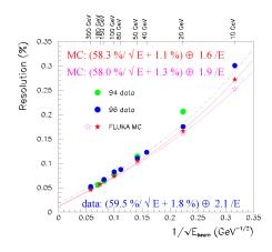
**FIGURE 17.** Fractional energy resolution as a function of beam momentum for the ATLAS combined calorimeter set-up. Two data sets (dots) correspond to two data takings[49, 50]. Stars: FLUKA simulations with two different preshower reconstruction algorithms.
