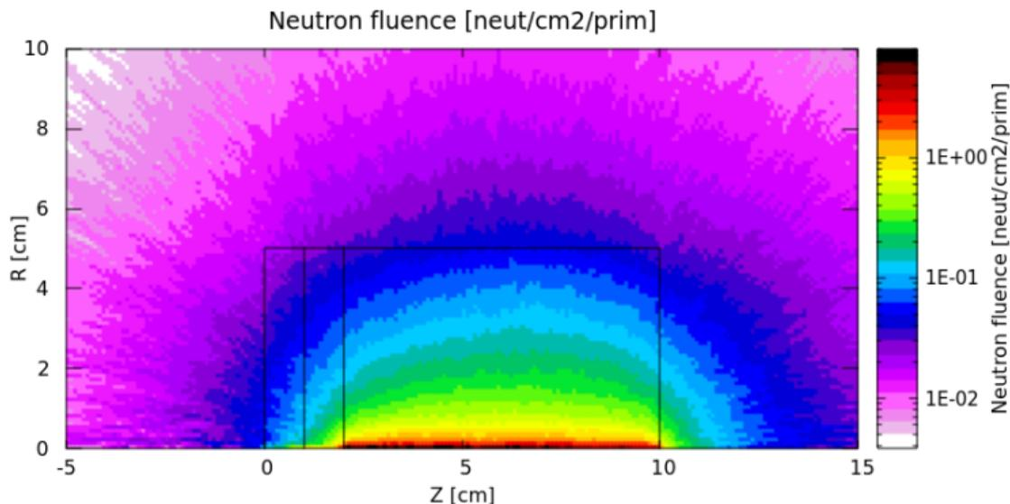
Same for **WHAT(2)** = HAD-CHAR: Charged hadron fluence from a 3.5 GeV proton beam hitting at [0., 0., 0.] directed along z. Results are normalized to **charged hadrons/cm<sup>2</sup> per primary**
