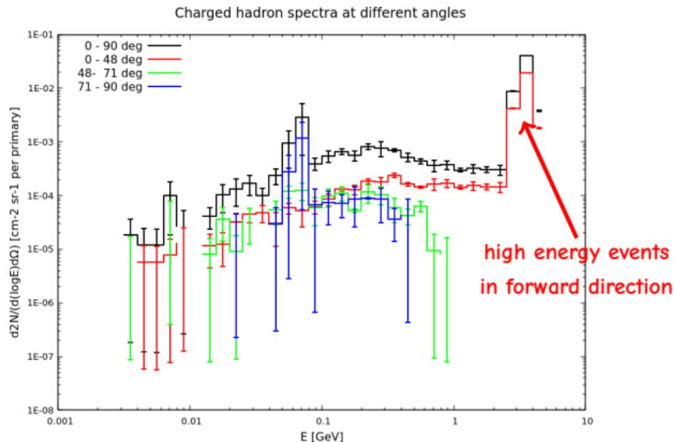
**USRTRK** calculates **differential fluence** as a function of **energy** by scoring track-length in a given region. Results are normalized to  $\text{GeV}^{-1} \text{cm}^{-2}$  per primary particle if the region volume is provided (otherwise should be intended as  $\text{GeV}^{-1} \text{cm}$  per primary particle, i.e. differential track-length). For all **SDUMs** except EN-NUCL and ENERGY:
