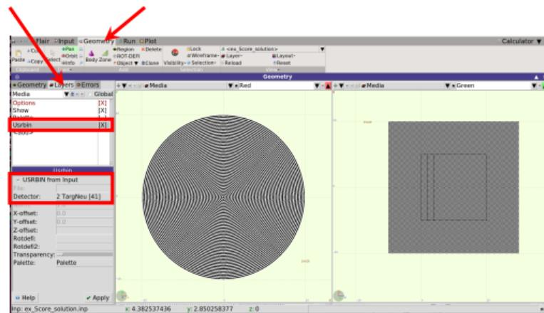
After you ran the example (next slide), deselect "USBIN from Input", and instead select the \*.bnn-file and plot the results inside the FLAIR Geometry-Menu.
