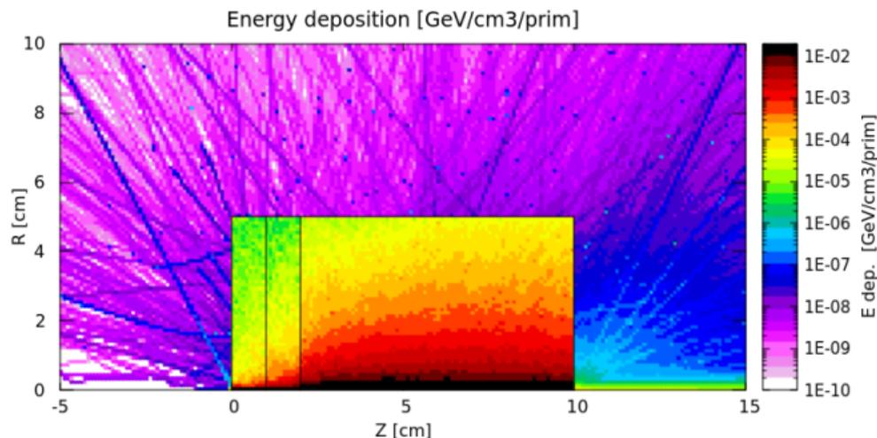
This plot is a 2D projection of a 3D structure → the result is averaged over the 3<sup>rd</sup> coordinate. Projection limits can be set in FLAIR.
