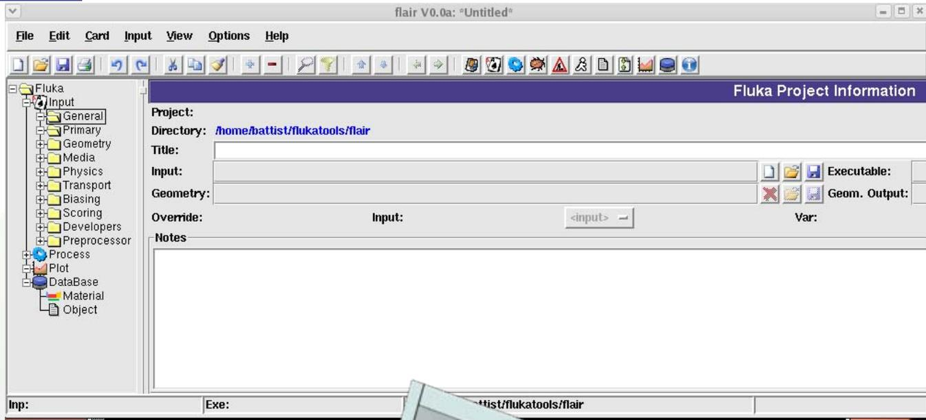
A FLUKA run can be managed through a graphical interface. Here is an example using python + Tk (**FLAIR**, V.Vlachoudis, CERN)
