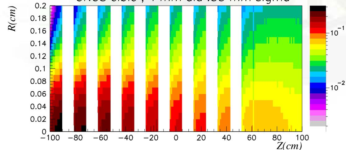
Muons in muon pits: horiz. distribution for beam alignment
