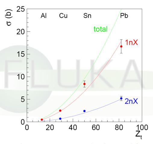
Electromagnetic dissociation cross sections (total, 1nX, 2nX) for 30GeV/n Pb ions on Al, Cu, Sn, and Pb targets.
