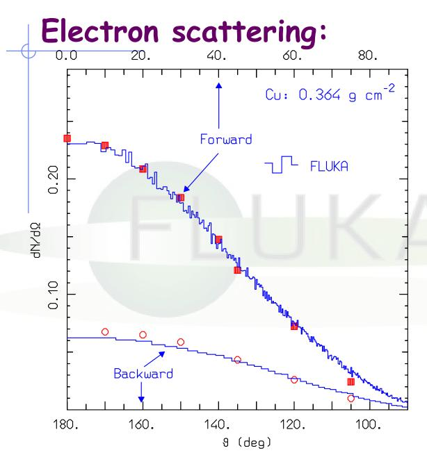
Transmitted (forward) and backscattered (backward) electron angular distributions for 1.75 MeV electrons on a 0.364 g/cm<sup>2</sup> thick Copper foil Measured (dots) and simulated (histos) data
