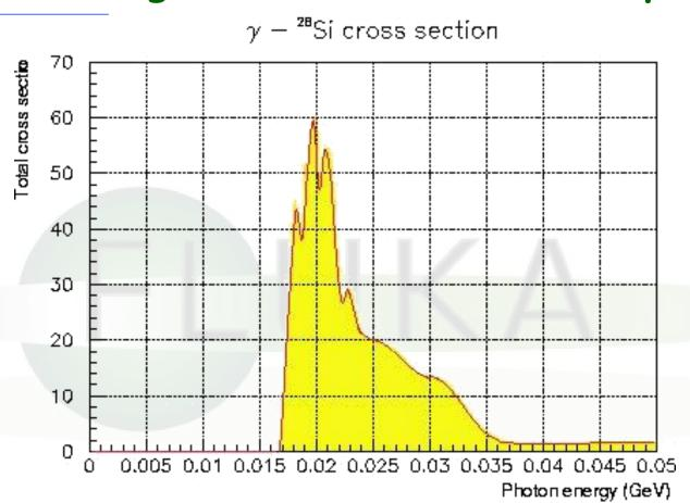
Left: <sup>28</sup>Si(g,tot) as recorded in FLUKA database, 8 interval Bezier fit as used for the Electromagnetic Dissociation event generator.
