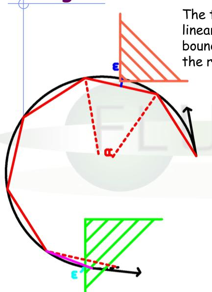
The true step (black) is approximated by linear sub-steps. Sub-step length and boundary crossing iteration are governed by the required tracking precision
