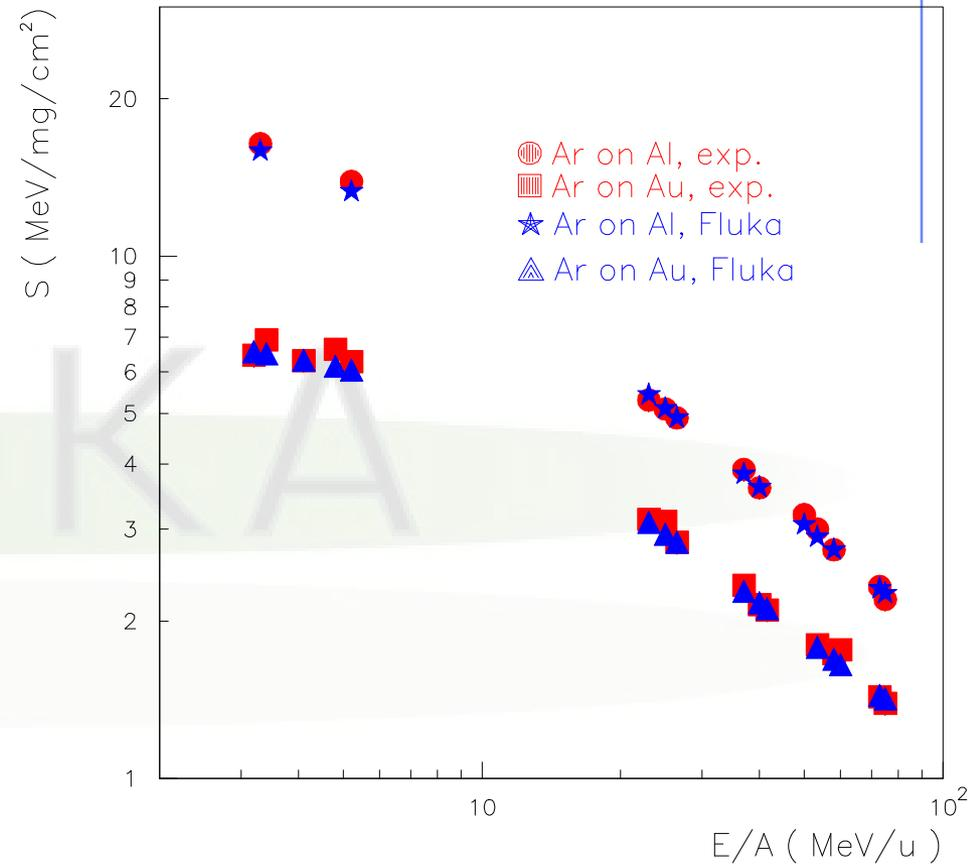
Comparison of experimental (R.Bimbot, NIMB69 (1992) 1) (red) and FLUKA (blue) stopping powers of Argon and Uranium ions in different materials and at different energies.
