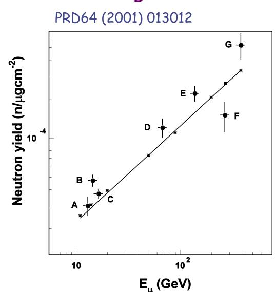
Neutron production rate as a function of muon energy
