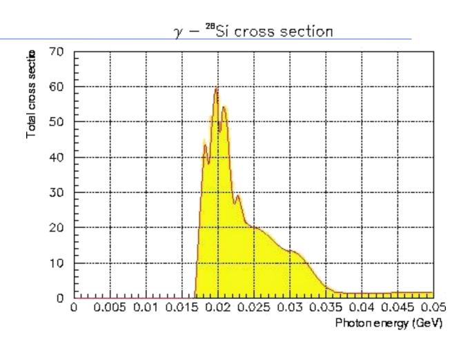
$^{28}$ Si( $\gamma$ ,tot) as recorded in FLUKA database, 8 interval Bezier fit as used for the Electromagnetic Dissociation event generator.
