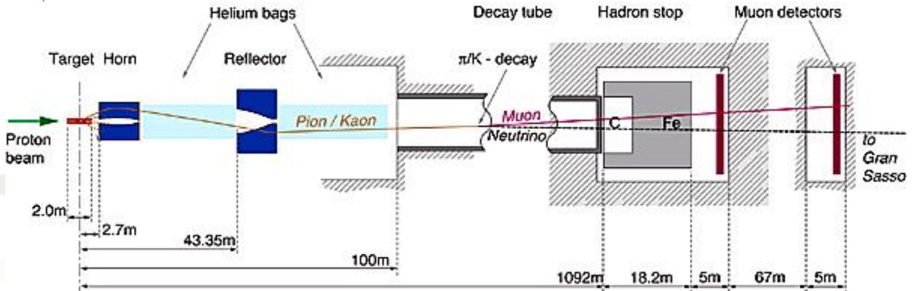
The two magnetic lenses (blue in the sketch) align positive mesons towards the Decay tunnel, so that neutrinos from the decay are directed to Gran Sasso, 730~km away
