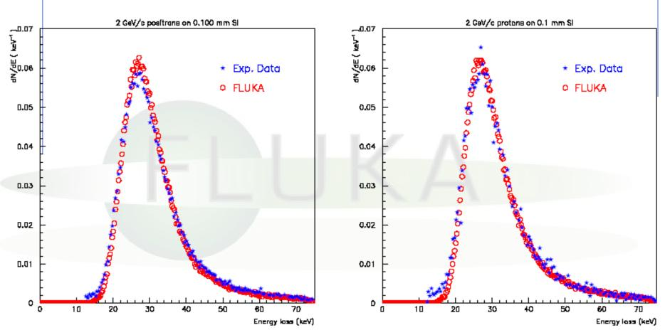
Experimental 1 and calculated energy loss distributions for 2 GeV/c positrons (left) and protons (right) traversing 100µm of Si J.Bak et al. NPB288, 681 (1987)
