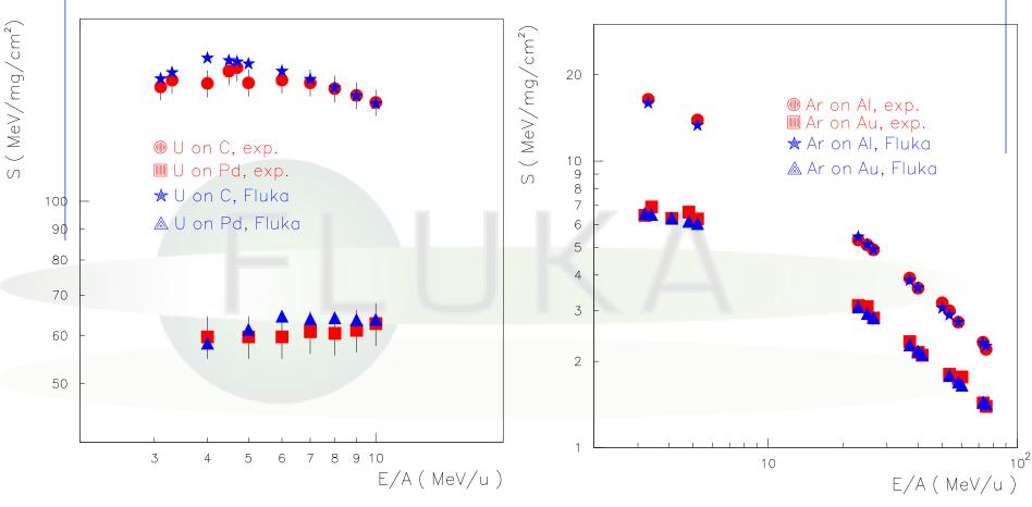
Comparison of experimental (R.Bimbot, NIMB69 (1992) 1) (red) and FLUKA (blue) stopping powers of Argon and Uranium ions in different materials and at different energies.
