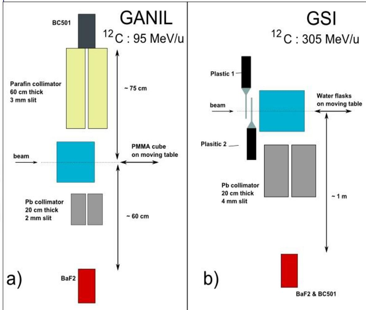
Prompt photons measured during irradiation of water and PMMA phantoms with C ions.
