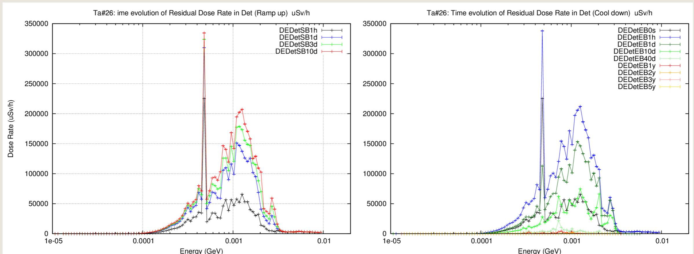
Detector placed 1 m away from the target (1m long x 10 cm thick)
