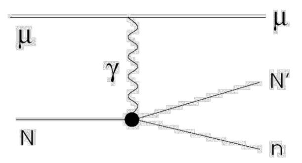
Schematic view of a  $\mu$  hadronic interaction. The interaction is mediated by a virtual photon. The final state can be more complex
