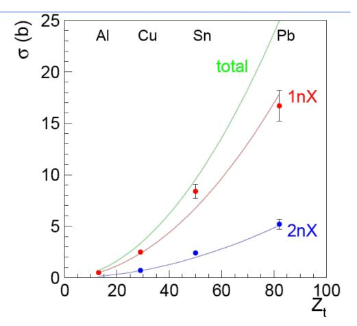
Electromagnetic dissociation cross sections (total, 1nX, 2nX) for 30GeV/n Pb ions on Al, Cu, Sn, and Pb targets.
