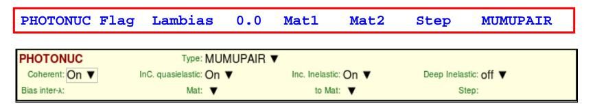
Flag controls activation of interactions, with the possibility to select a subset of the photomuon mechanisms (coherent, incoherent, inelastic...) Biasing of photomuon production can be done directly with this card, setting WHAT(2)
