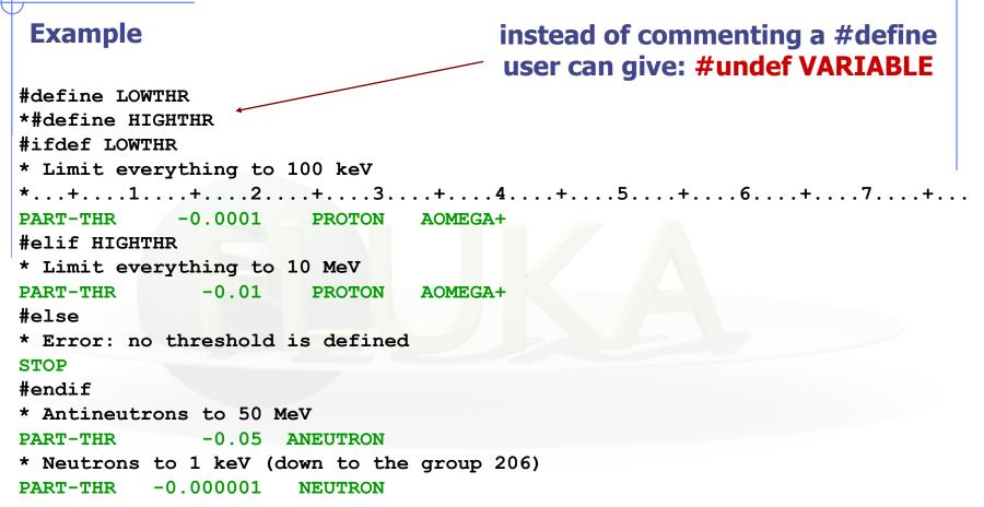
Depending on which threshold is selected (LOWTHR or HIGHTRH) the respective PART-THR is used (except for neutrons and antineutrons)
