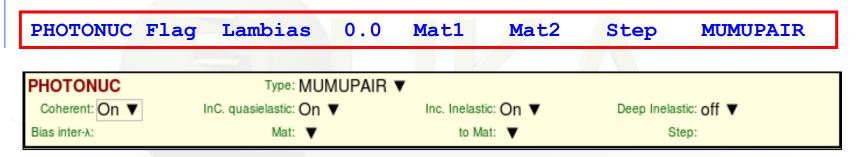
Flag controls activation of interactions, with the possibility to select a subset of the photonuclear mechanisms
