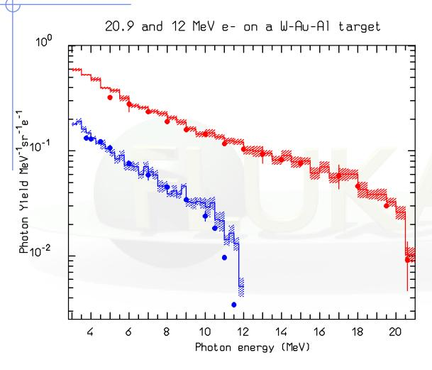
12 and 20.9 MeV electrons on a W-Au-Al target, bremsstrahlung photon spectra in the forward direction measured (dots) and simulated (histos)
