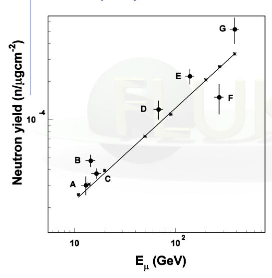
Neutron production rate as a function of muon energy
