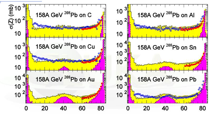
Fragment charge cross section for 158 AGeV Pb ions on various targets. Data (symbols) from NPA662, 207 (2000), NPA707, 513 (2002) (blue circles) and from C.Scheidenberger et al. PRC70, 014902 (2004), (red squares), yellow histos are FLUKA (with DPMJET-III) predictions: purple histos are the electromagnetic dissociation contribution
