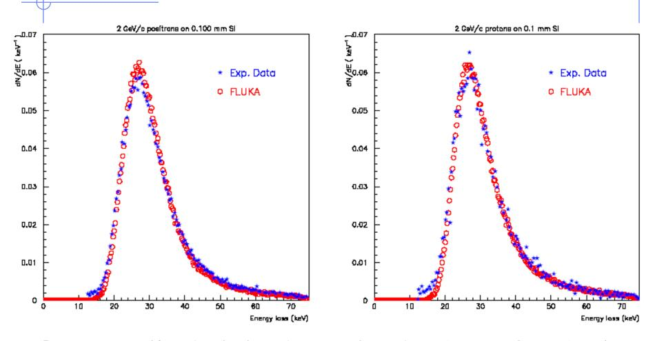
Experimental  $^1$  and calculated energy loss distributions for 2 GeV/c positrons (left) and protons (right) traversing 100  $\mu$ m of Si
