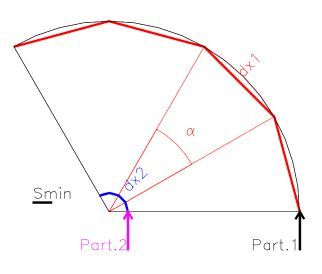
Particle 1: the sub-step corresponding to  $\alpha$  is > Smin -> accept Particle 2: the sub-step corresponding to  $\alpha$  is < Smin -> increase  $\alpha$
