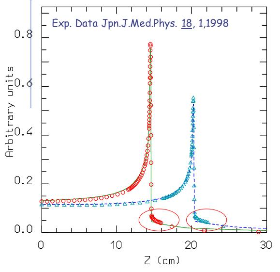
Dose vs depth distribution for 270 and 330 MeV/n  $^{12}C$  ions on a water phantom.
