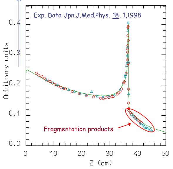
Dose vs depth distribution for 670 MeV/n <sup>20</sup>Ne ions on a water phantom.
