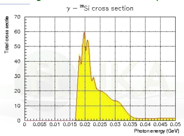
Left:  ${}^{28}Si(\gamma,tot)$  as recorded in FLUKA database, 8 interval Bezier fit as used for the Electromagnetic Dissociation event generator.
