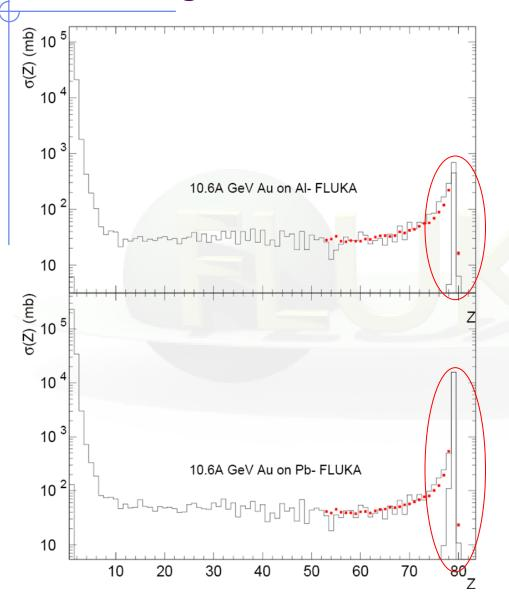
Fragment charge cross sections for 10.6 GeV/n Au ions on Al and Pb.
