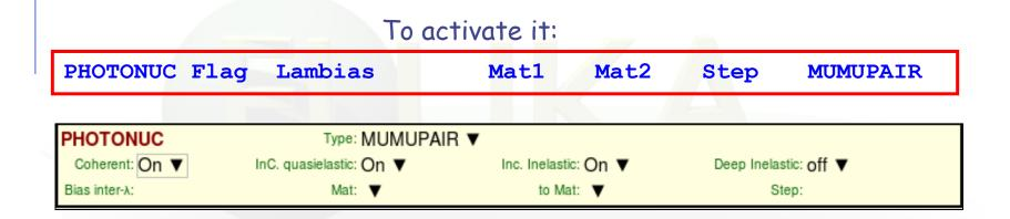
Flag controls activation of interactions, with the possibility to select a subset of the photonuclear mechanisms
