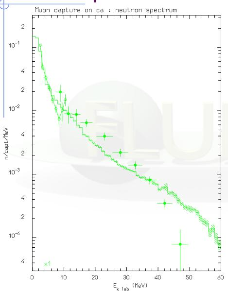
capture on Calcium Dots: experimental data (Columbia Univ. rep. NEVIS-172 (1969), Phys. ReV. C7, 1037 (1973), Yad. Fiz. 14, 624 (1972) histograms: FLUKA calculations **Emitted:** 0.62 neutrons/capture 0.27 protons/capture
