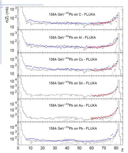
Fragment charge cross sections for 158GeV/n Pb ions on various targets.
