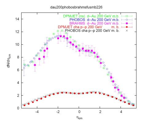
Pseudorapidity distribution of charged hadrons produced in minimum bias d-Au and p-p collisions at a c.m. energy of 200GeV/A.
