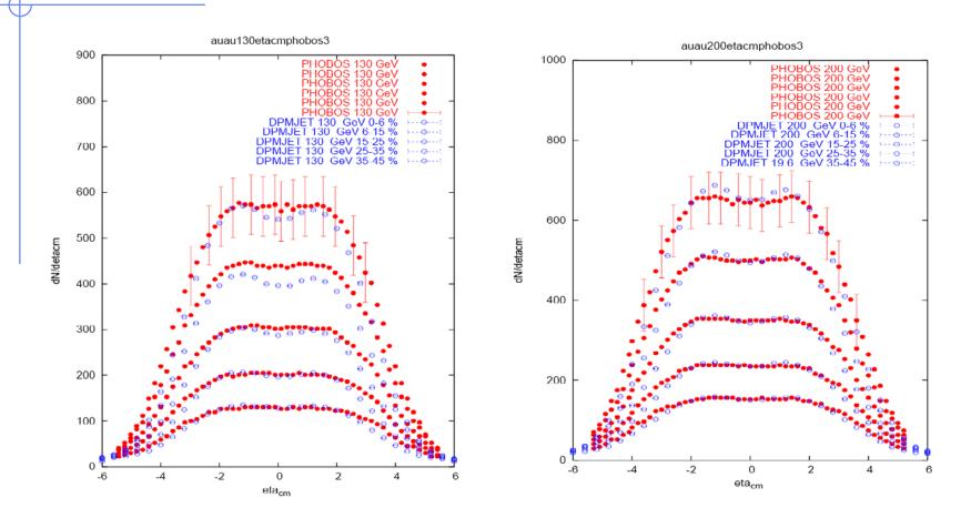
Pseudorapidity distribution of charged hadrons produced in Au-Au collisions at a c.m. energy of 130GeV/A (left) and 200GeV/A (right) for different ranges of centralities.
