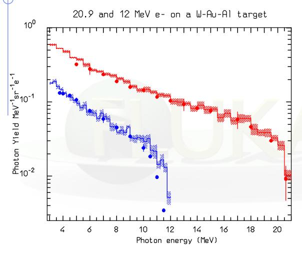
12 and 20.9 MeV electrons on a W-Au-Al target, bremsstrahlung photon spectra in the forward direction measured (dots) and simulated (histos)
