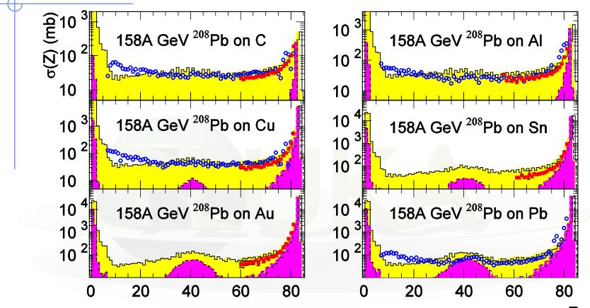
Fragment charge cross section for 158 AGeV Pb ions on various Z targets. Data (symbols) from NPA662, 207 (2000), NPA707, 513 (2002) (blue circles) and from C.Scheidenberger et al. PRC70, 014902 (2004), (red squares), *yellow* histos are FLUKA (with DPMJET-III) predictions: *purple* histos are the electromagnetic dissociation contribution
