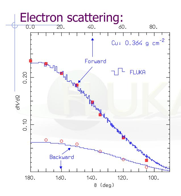
Transmitted (forward) and backscattered (backward) electron angular distributions for 1.75 MeV electrons on a  $0.364 \, \text{g/cm}^2$ thick Copper foil Measured (dots) and simulated (histos) data
