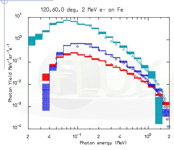
2 MeV electrons on Iron, Bremsstrahlung photon spectra measured (dots) and simulated (histos) at three different angles
