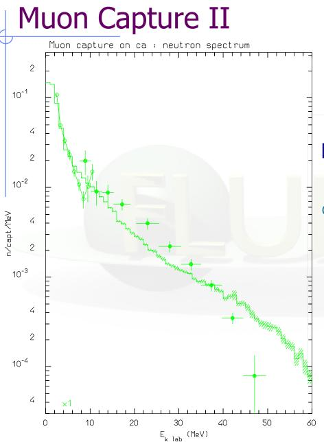
capture on Calcium Dots: experimental data (Columbia Univ. rep. NEVIS-172 (1969), Phys. ReV. C7, 1037 (1973), Yad. Fiz. 14, 624 (1972) ) histograms: FLUKA calculations Emitted: 0.62 neutrons/capture 0.27 protons/capture
