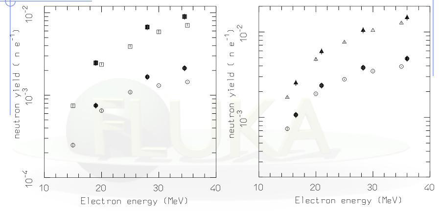
Yield of neutrons per incident electron as a function of initial e<sup>-</sup> energy. Open symbols: FLUKA, closed symbols: experimental data (Barber and George, Phys. Rev. 116, 1551-1559 (1959)) Left: Pb, 1.01  $X_0$  (lower points) and 5.93  $X_0$  (upper) Right: U, 1.14 and 3.46  $X_0$
